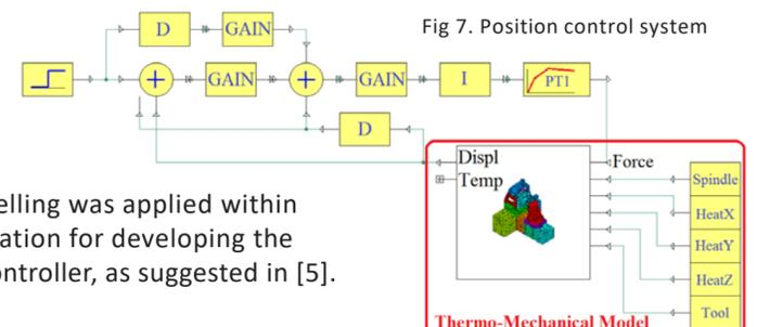
Reduced order modelling was applied within a system-level simulation for developing the real-time position controller, as suggested in [5].
