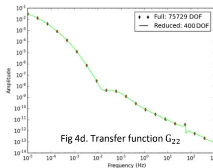
The strongly coupled machine tool model suffers from different time constants for the structural dynamics and heat transfer behavior. The reduced model has to match the frequency range from 0Hz to 10Hz (thermal expansion) as well as the range from 1Hz to 1000Hz (dynamics).
