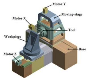
Fig 2. Structure of the machine tool model
