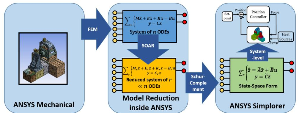
Fig 3. Workflow for the system-level simulation of the machine tool model
