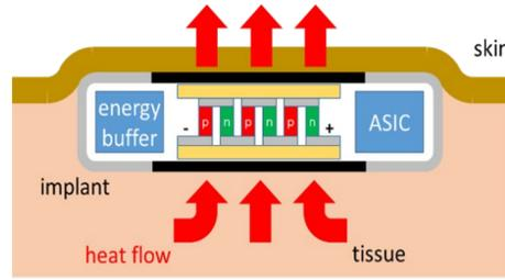
Fig. 1. Implant with thermoelectric energy conversion powered by flow of body heat
