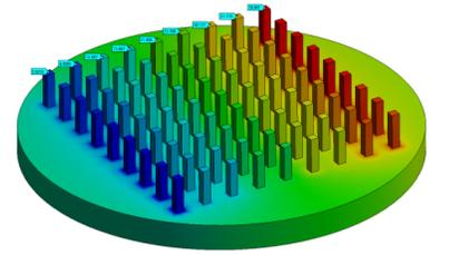
Fig. 2. Electric potential across 81 thermocouple legs of bismuth telluride.
