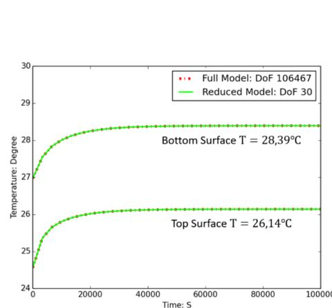
Fig. 6. Temperature comparison between full and reduced models at top and bottom surface of the center thermocouple leg in TEG model.
