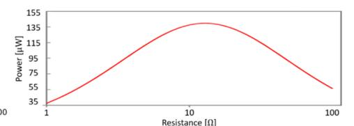
Fig. 8. Power dissipated in load resistor for different load resistance values.
