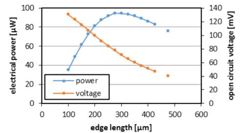
Fig. 4. Influence of the leg edge length on electrical power output and temperature difference in TEG
