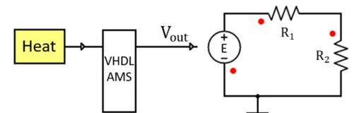
Fig. 7. Co-simulation setup with VHDL-model for transient thermal analysis of power output
