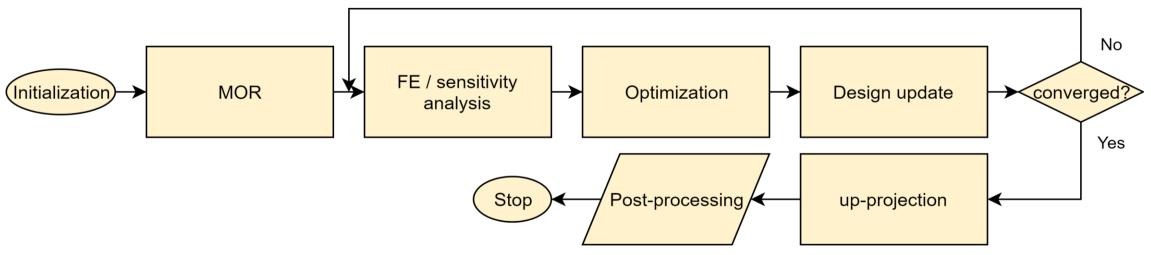
Flow chart of a MOR-accelerated TO where the optimization itself is actually performed on a reduced order model. The optimal full order realization can be than be obtained by up-projection. This approach is significantly more efficient than 'on-the-fly' approaches as MOR is performed offline.
