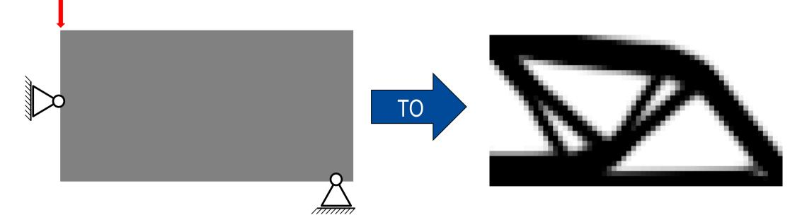
Compliance minimization using TO. Starting from a full block with 50% density, TO manipulates the material distribution to obtain a structure with minimal compliance for the given load case (Algorithm taken from [3]).
